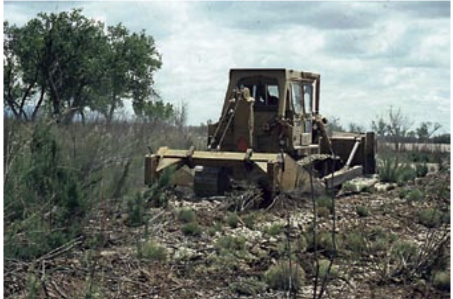
Figure 8. Root plowing of saltcedar on Bosque del Apache National Wildlife Refuge
